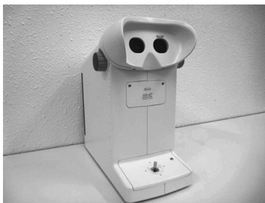
Figure 3 Motion visual acuity tester (AS-4F, Kowa, Tokyo)
