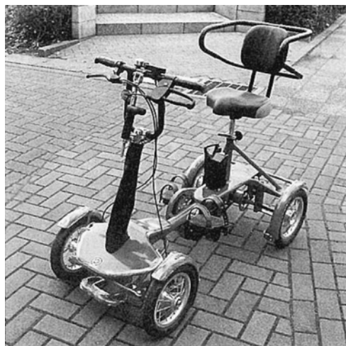
図 1 A four-wheel electric power-assisted personal mobility
